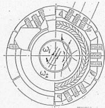
Scheme showing how to implement two types of RMF in one inductor
